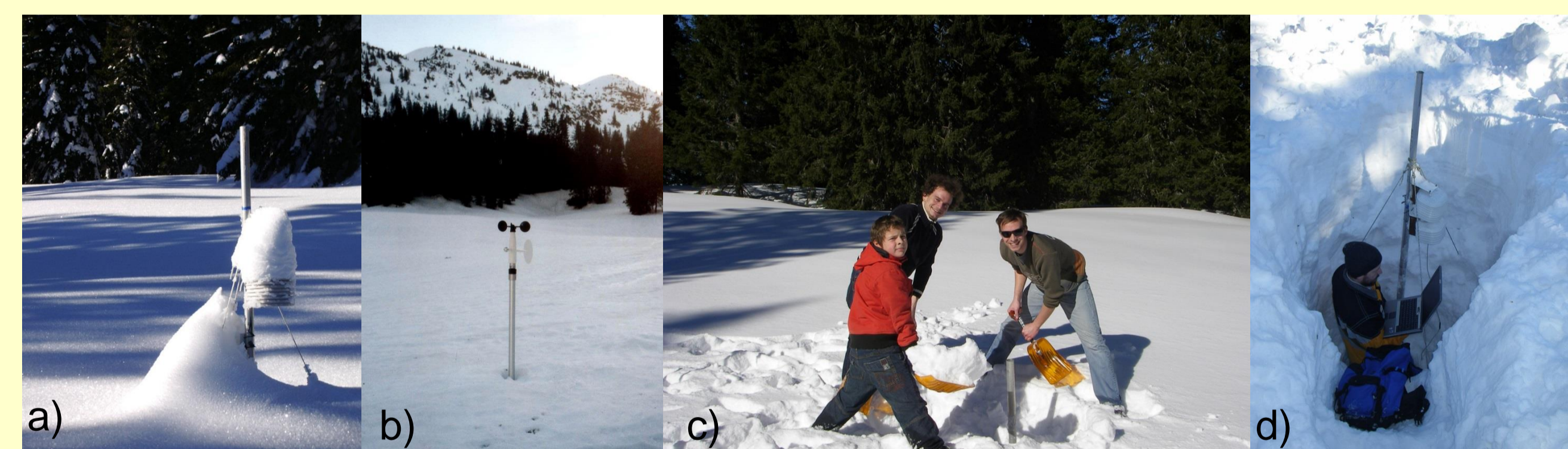
Figure 1: Illustration of measurements problems in snow rich and remote mountainous regions. a) Temperature sensor almost snow covered; b) Wind anemometer of weather station only about 50cm above snow surface; c) students are digging out the station; d) data download from the snow covered loggers.
