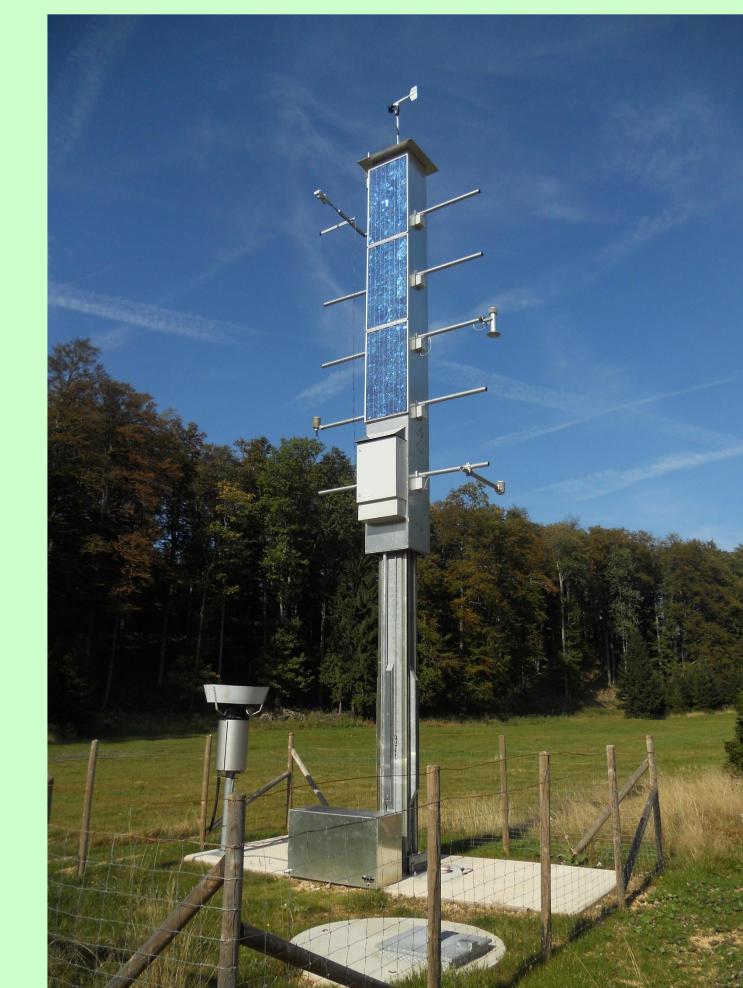
Figure 7: METLIFT at its maximum lifting height of 4m.
