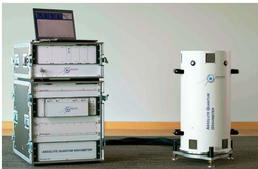
Figure 3. The Muquans absolute quantum gravimeter, based on laser-cooled atoms. Credit: Muquans.
