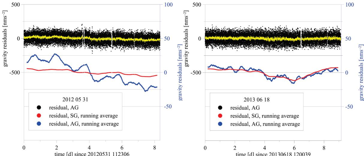
Fig. 3. Calibration experiments at CO in May/June 2012 (left) and in June 2013 (right). In contrast to 2013, the AG Rb-oscillator was exposed to abnormal helium gas in 2012. Black: single AG drops, yellow: their moving average (21 samples, yellow), red: SG residuals (moving average, 1001 samples), blue: AG drops (moving average, 1001 samples).
