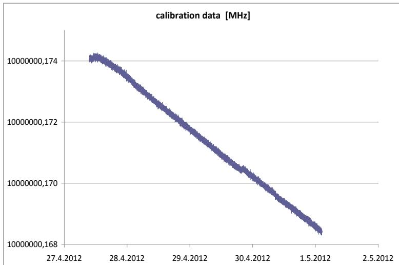
Fig. 1. Drift rate of the Rb-oscillator (about 5 mHz in 4 days), after storing the AG for a few months at CO.
