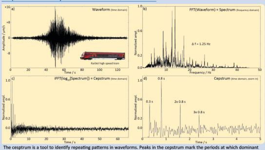
patters in the waveforms repeat. This example is for the Railjet high-speed train. a) Raw waveform in units of velocity. b) Spectrum of the waveform. c) Cepstrum of the waveform. d) Zoom onto the main peaks in the cepstrum. The highest peak in the cepstrum (0.8 s) corresponds to a frequency spacing of  $\Delta f = 1/0.8 = 1.25$  Hz. The peaks at longer periods are higher orders of the main peak. A patch of signal repeating each 0.8 s is also visible in the waveforms when zooming in.
