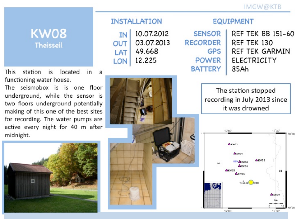
Figure A8. Station KW08 technical information.
