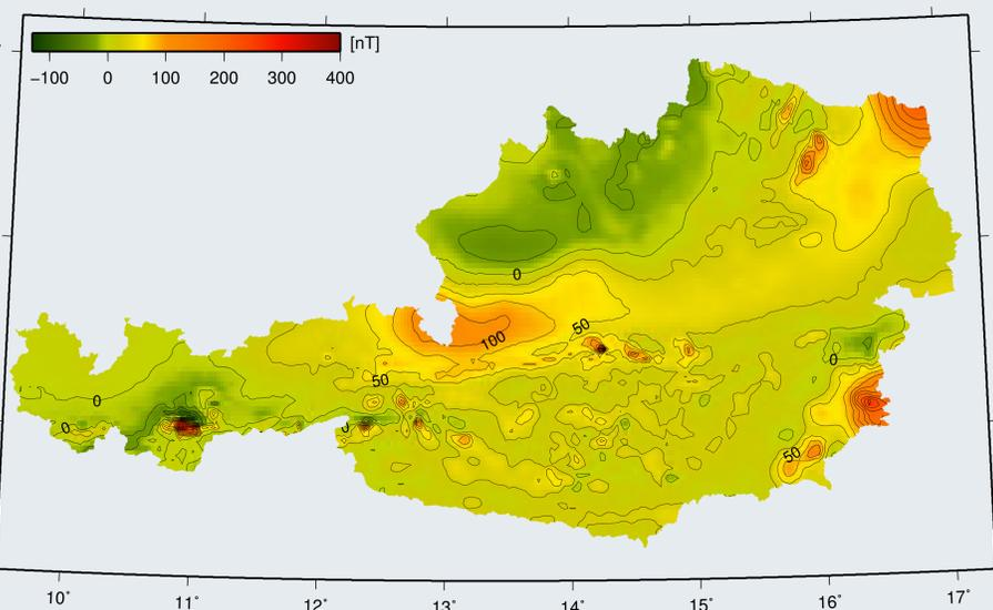
**Fig. 3:** Magnetic residual field derived from aerial surveys (1977-1982) continued to a common height of 3000 m above sea level (Blaumoser, 1991).
