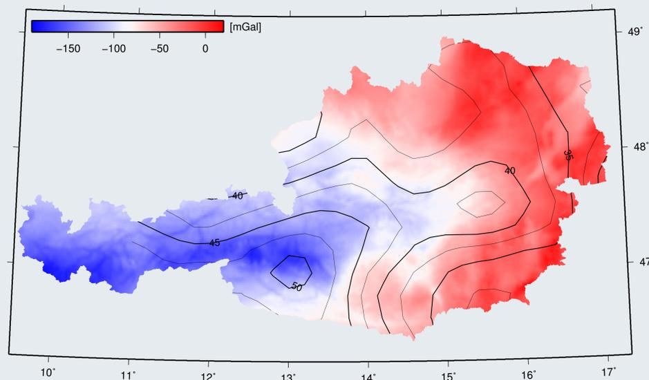
**Fig. 4:** Bouguer Anomaly map based on the orthometric height system (Meurers & Ruess, 2009) and contour lines depict Moho depths in km (Behm et al., 2007).
